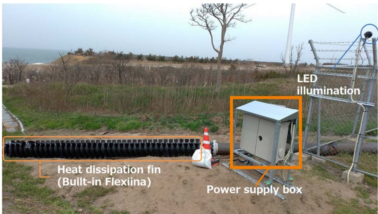
Fig.3 Demonstration experiment at JX Nippon Oil & Gas Exploration Corporation
